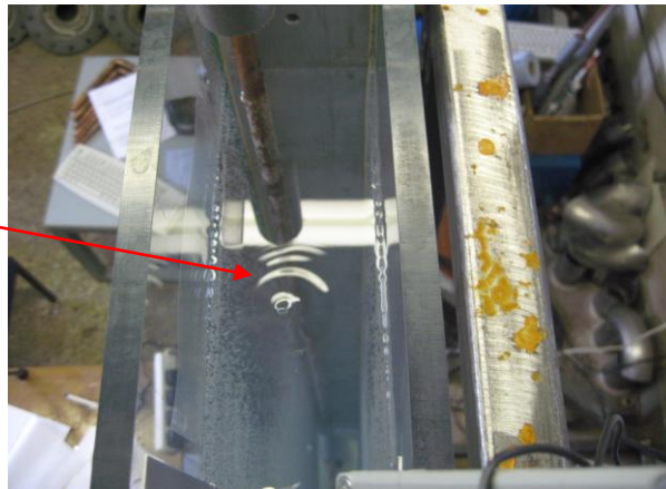
Figure 6-20: Free surface distortion when bubble hits the free surface
