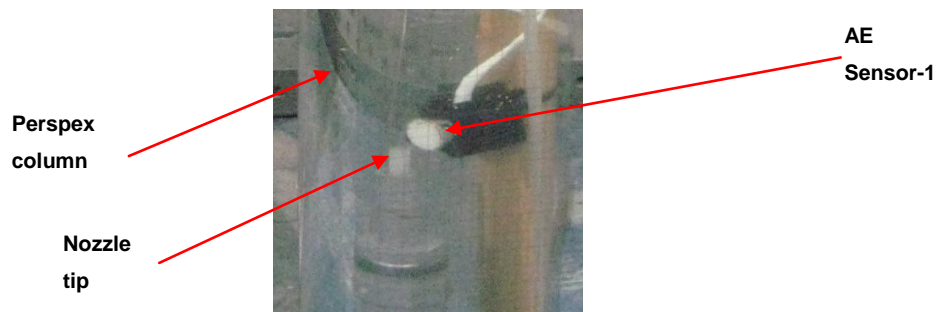
Figure 4-3: Picture of nozzle and AE sensor-1
