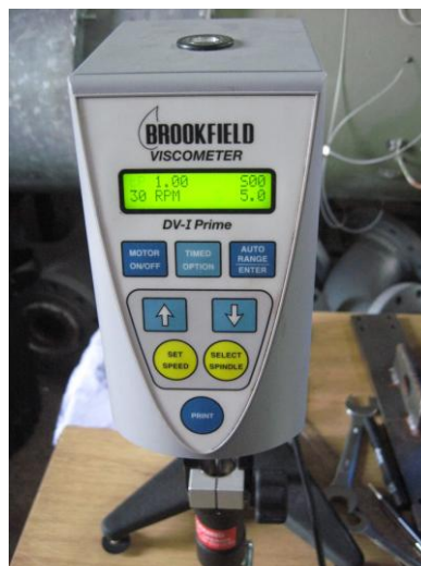
Figure 4-6: Tap water measured by BROOKFIELD, DV-I Prime viscometer
