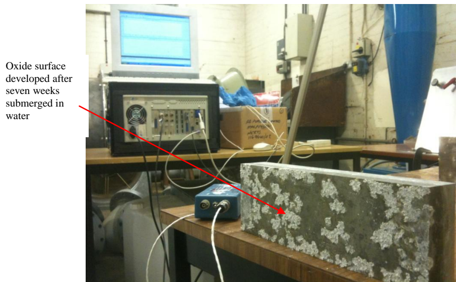
Figure 3: Surface degradation (oxide) developed after seven weeks submerged in water
