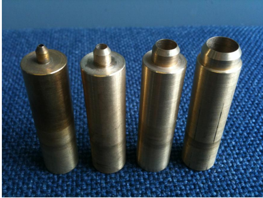
Figure 4-8: Four different sizes of nozzle used in the advanced test rig made of brass and cone-shaped at each nozzle's tip
