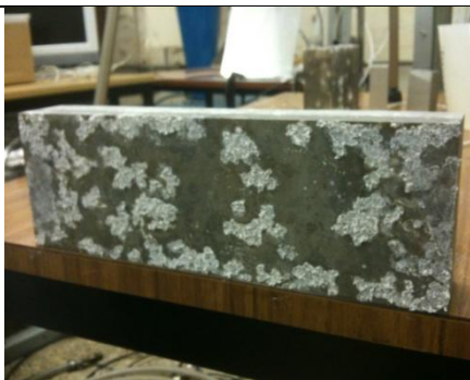
(d) Surface after seven weeks half submerged in water
