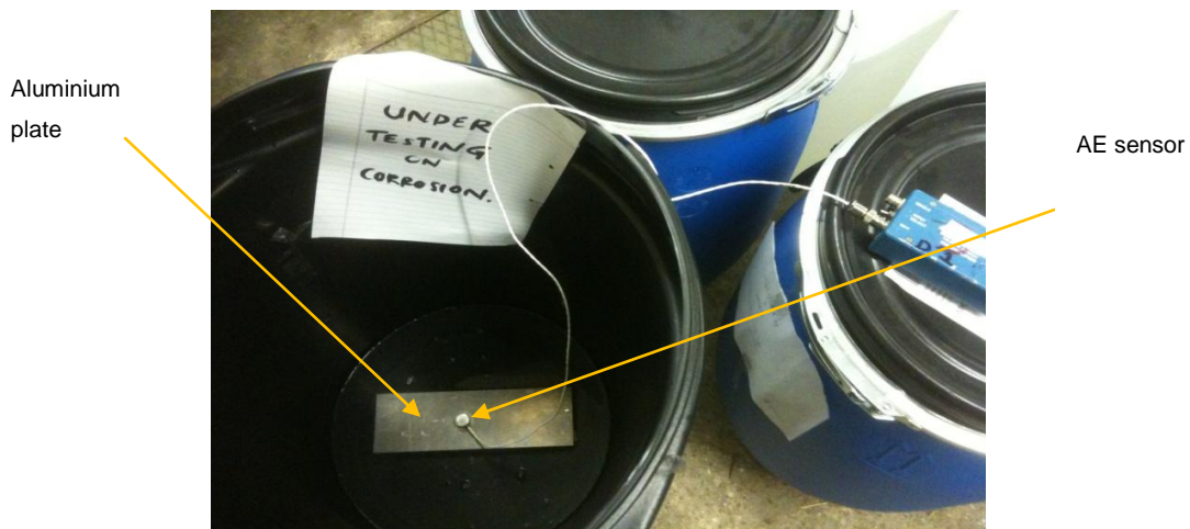
Figure 1: Aluminium plate submerged half its thickness in water
