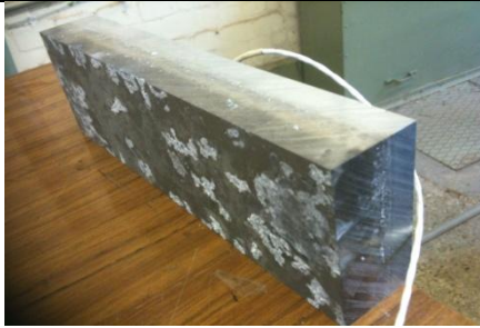
(b) Surface after two weeks submerged in water
