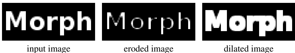
Figure 5.2: Grey scale erosion and dilation
