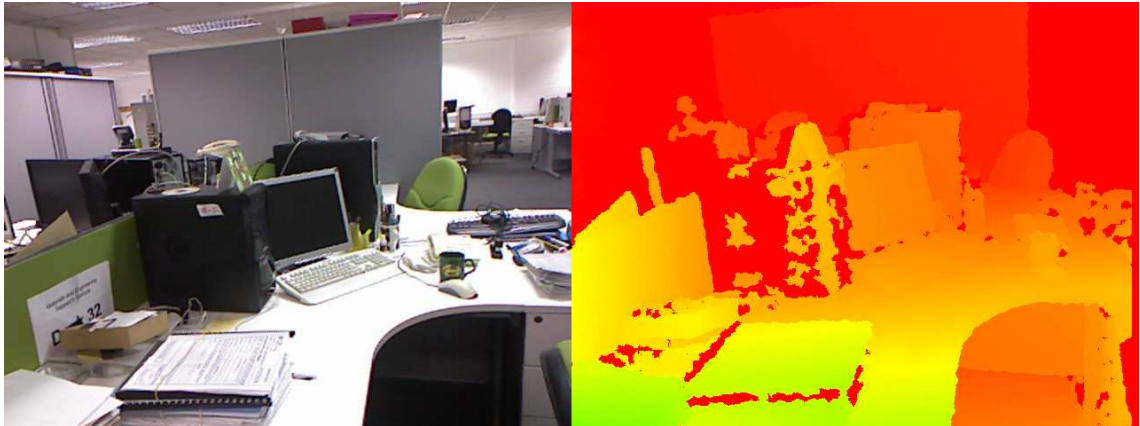
Figure 4.15: RGB- and depth-image acquired with an RGBD sensor
