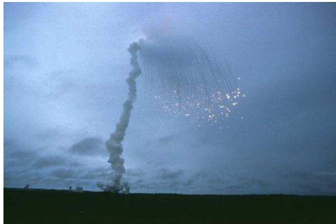
Figure 1.7: Ariane 5 disaster caused by numerical overflow
