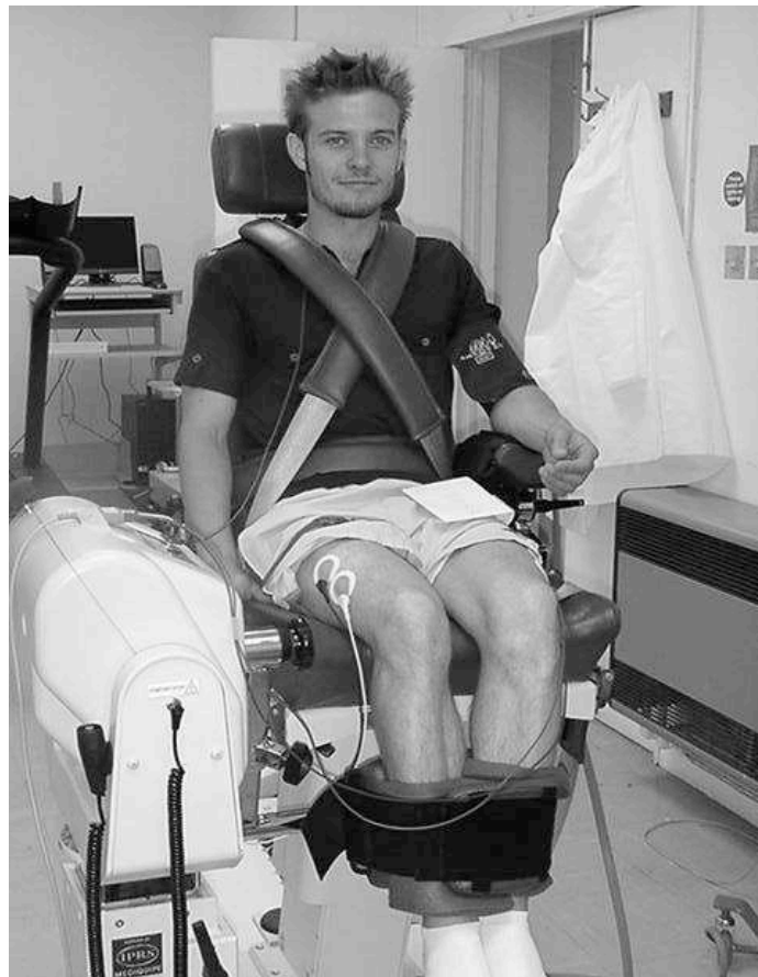
Figure 2.2. Participant position on the dynamometer
