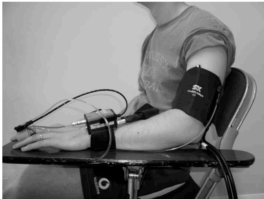
Figure 2.7. Upper arm cuff, microprocessor wrist block, finger cuff, and hydrostatic height sensor arrangement
