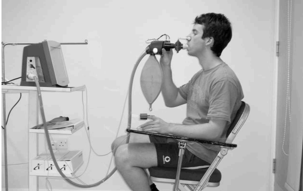
Figure 2.11. Resting cardiac output (Q) and stroke volume (SV) measurement with the Innocor device
