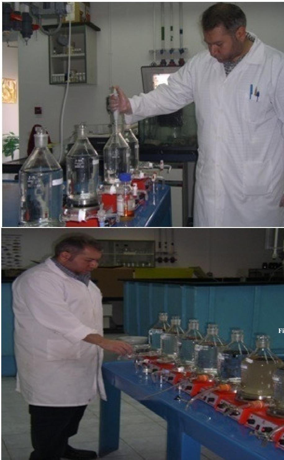
Figure 3-1: Preparation of Kuwait crude oil WAF and CE-WAF solutions in laboratory
