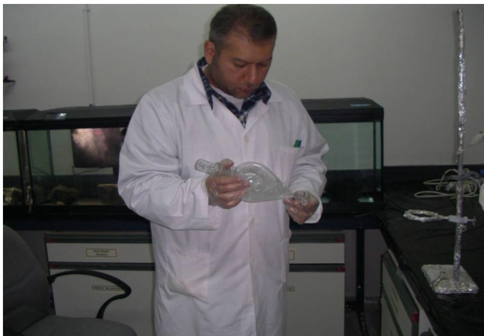
Figure 3-3: Chemical extraction of Kuwait crude oil WAF and CE-WAF with dichloromethane and collection of extracted solution
