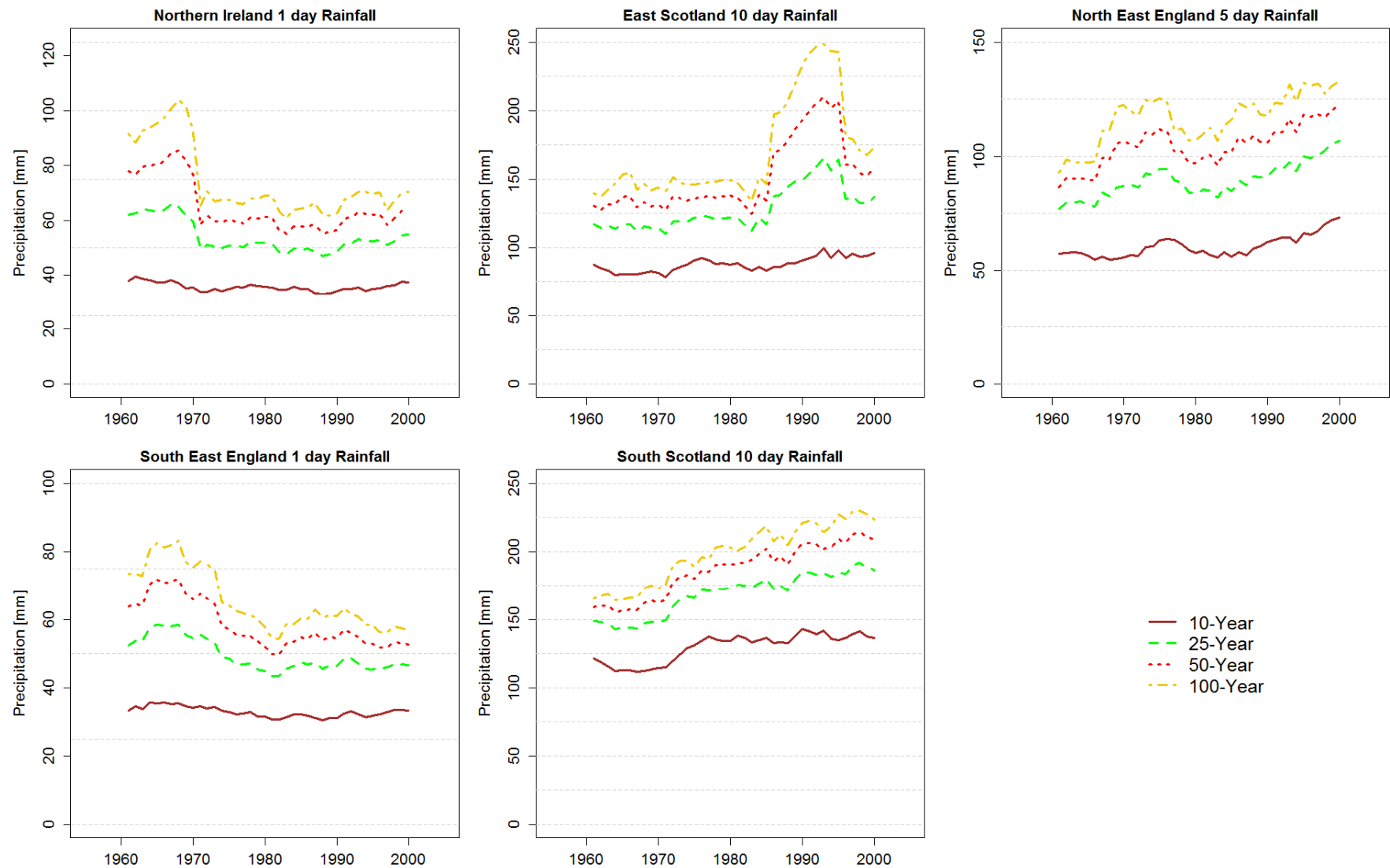
Figure 6-9 : Rolling decadal return period estimates fitted for 1961-2009: (a) NI region, 1-day; (b) ES region, 10-day; (c) NEE region, 5-day; (d) SEE region, 1-day; (e) SS region 10-day
