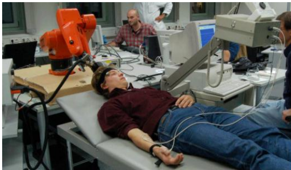
Figure 2-6 Application set up. The patient's head is tracked by a POLARIS camera (not visible) enabling the robot to compensate for head movements [Matthäus et al., 2006b]
