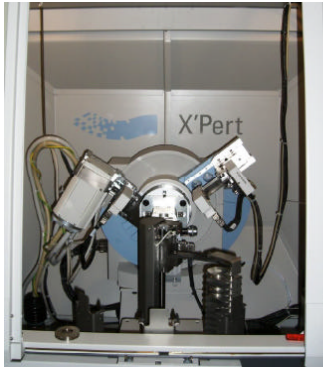
Figure 2: An X-ray diffractometer (Panalytical X'pert pro, Almelo, Netherlands).
