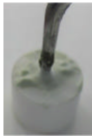
Figure 13: MTA slurry being treated with ultrasonic vibration.
