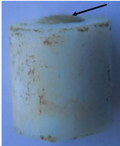
Figure 67: Uneven hemispherical expansion of MTA out of the end of a cylindrical mould that was exposed to WFH blood is shown by the arrow.
