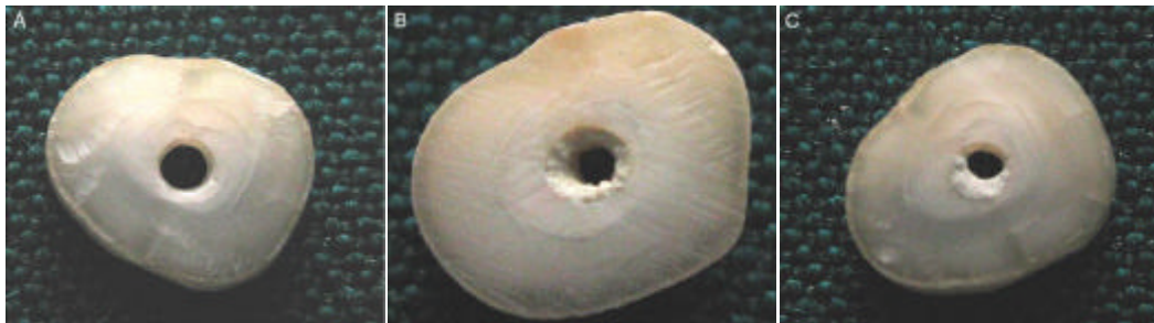
Figure 33: Various failure modes. (A) Adhesive failure; note the clean canal wall. (B) Cohesive failure within MTA. (C) Mixed failure; note the MTA residual inside the canal.
