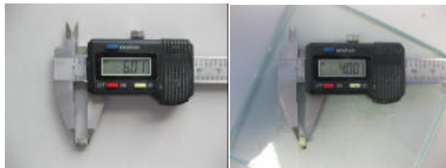
Figure 16: The dimensions of specimens were rechecked prior to the compressive test.
