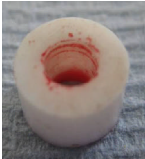
Figure 55: In the test groups, before placement of the MTA slurry, the inner walls of moulds were coated with WFH blood.
