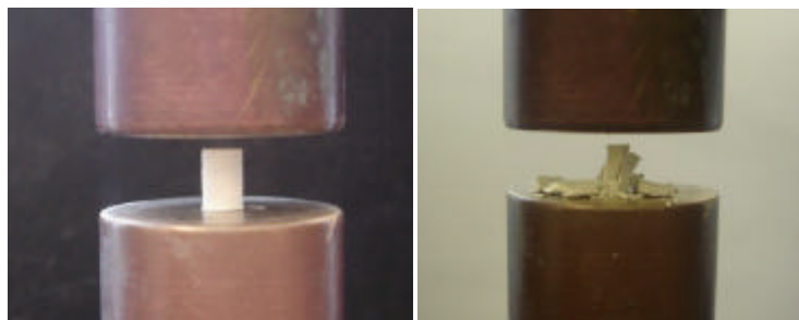
Figure 4: A tooth coloured ProRoot 2 MTA specimen during the compressive test using the universal testing machine.
