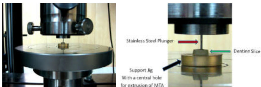
Figure 32: A cylindrical stainless steel plunger attached to the load cell of the universal testing machine loading on MTA inside a root section.
