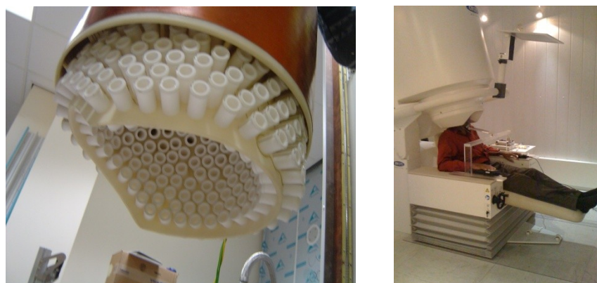
Figure 3.2. The MEG system A shows the 275 gradiometers in the MEG system (prior to install). B shows a subject in the MEG, during a tactile experiment. The subject is raised up into the helmet. A chin-rest is used for additional support
