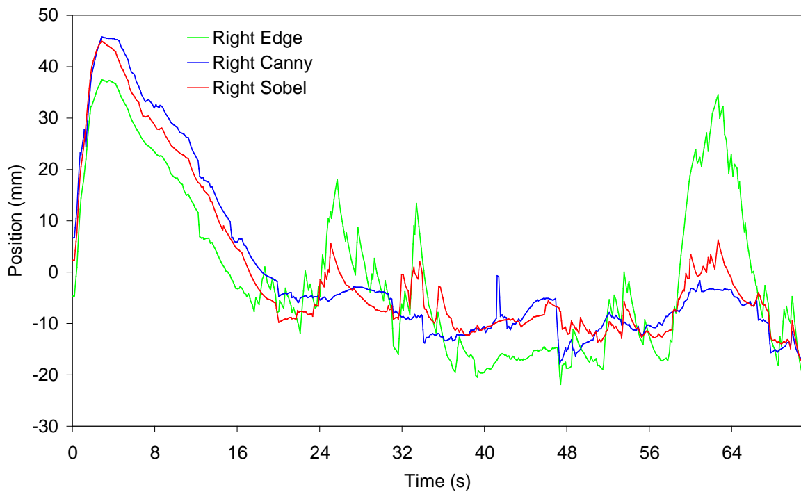
Figure 3.12: Comparison of image filters, right edge, low pass filter applied ( \alpha = 0.05 )
