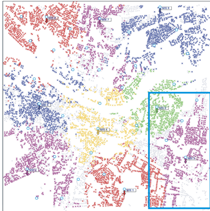
Figure 5.11: Base station '3' with capacity of 6 sectors
