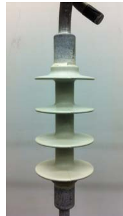
Polymeric insulator ready for laboratory test
