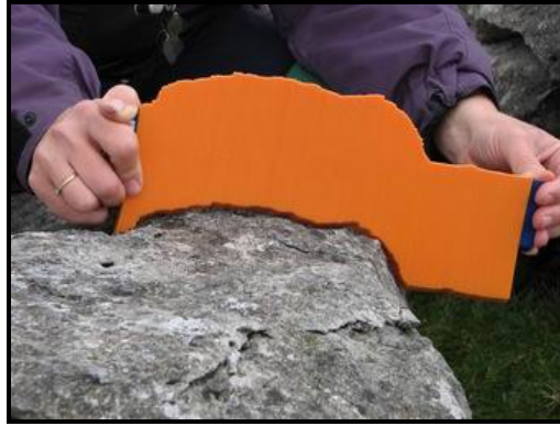
Figure 2-4: Carpenter's profile gauge, used to estimate the degree of roundness of the clint edge. The first three clints were measured at a uniform point and the profile recorded was then compared against Power's 'Scale of Roundness'.
