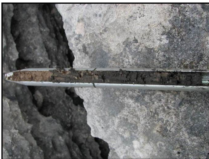
Figure 3-25: Variation in soil profile at Holmepark Fell (HRHPE).
