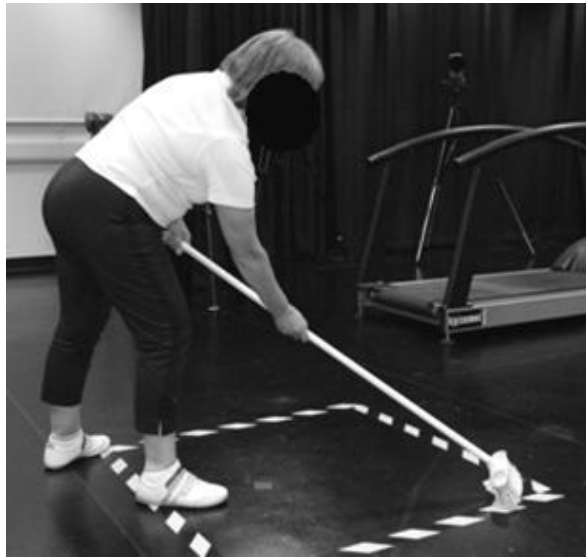
Figure 15. Sweeping. Participants were asked to sweep a 1 m 2 area of floor for one minute. Participants were required to reach to the edge of the marked area with each sweep. Determining a 1 m 2 floor area ensured participants reached the same distance (Jacobs, 2008; Mackinnon, 1999).
