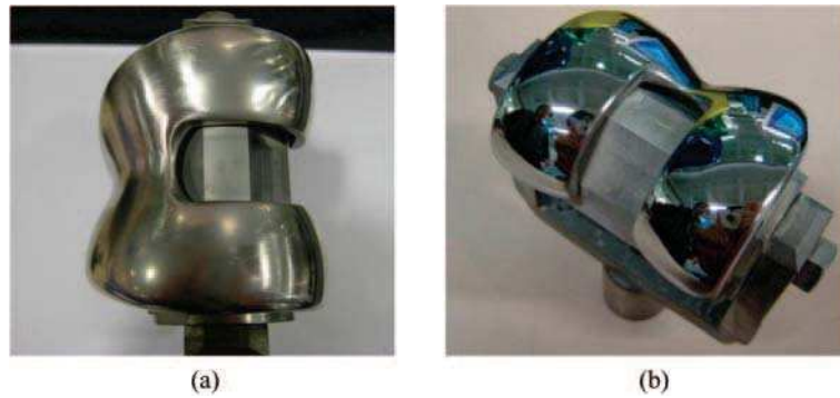
Fig. 17 Surface quality of the orthopaedic implant (a) before and (b) after polishing
