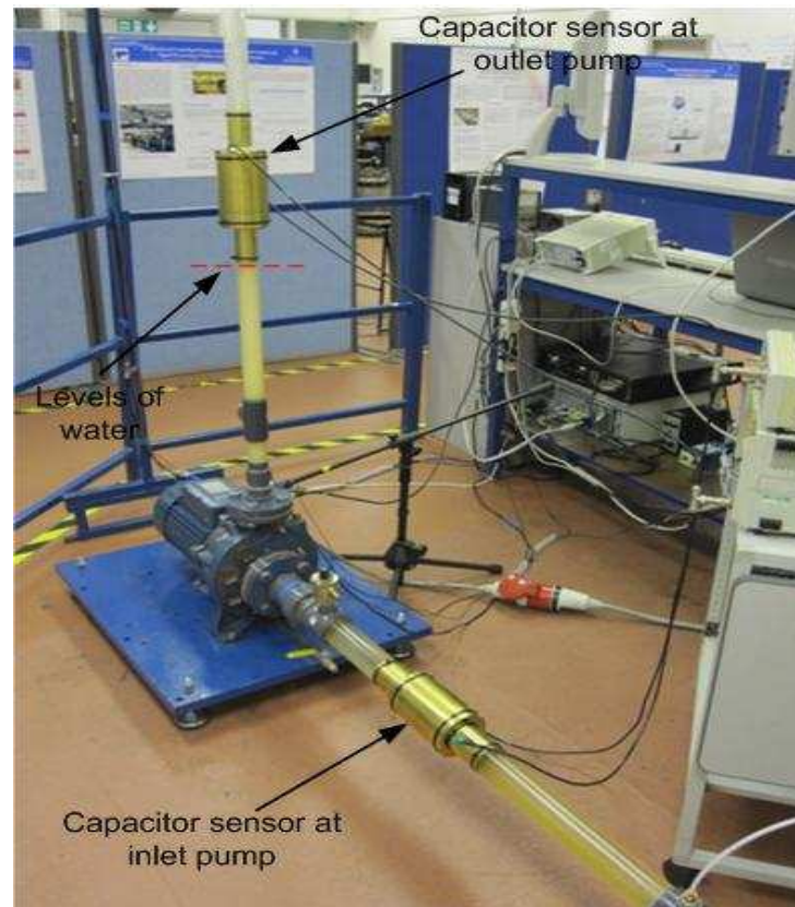
Figure 5-3 Capacitive sensors at inlet and outlet of the pump
