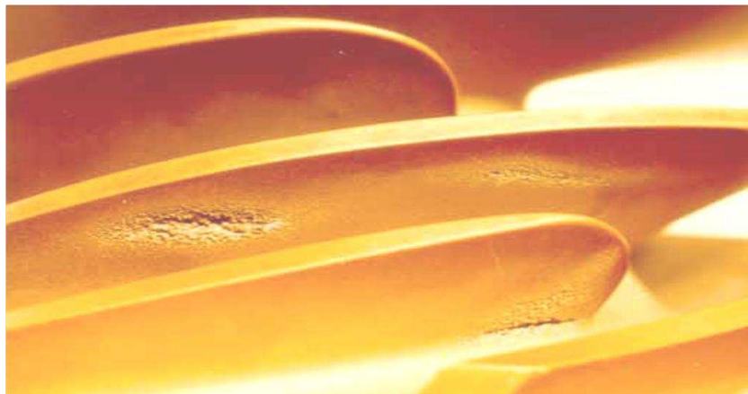
Figure 2-14 Cavitation damage on the blade of a closed impeller (Brennen, 1995)
