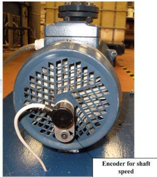
Figure 4-19 Position of encoder for shaft speed
