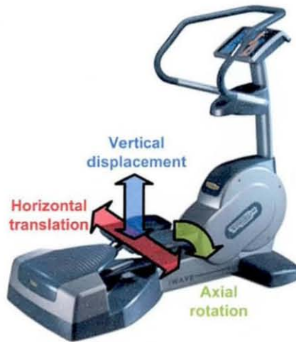
Figure 2.3: Operational movement planes offered by state of the art stepper devices.
