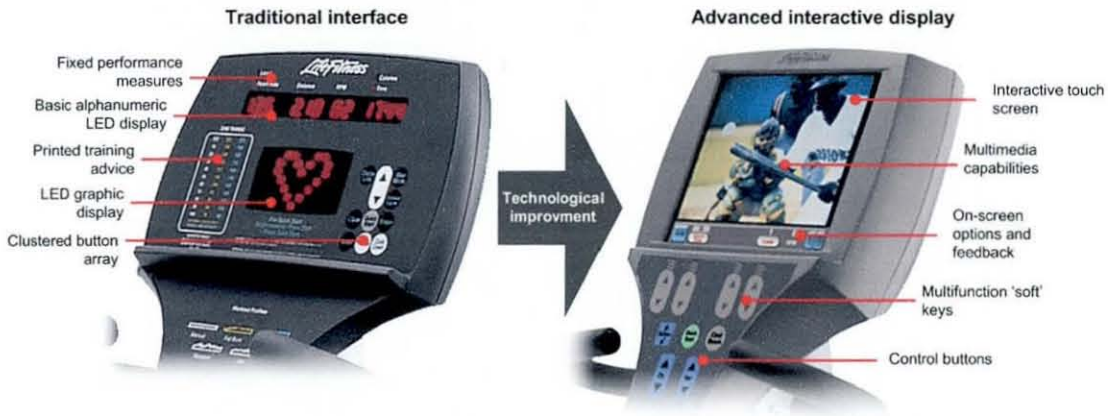
Figure 6.4: Existing aerobic equipment interfaces and key design features.
