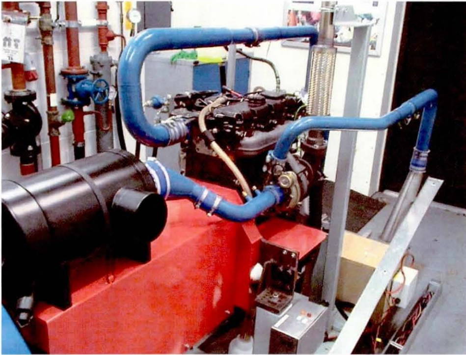
Figure 3.25. Photograph of the test engine; a Perkins 1100 series, 4 cylinder, 4.4 litre turbocharged, charge-cooled diesel engine.
