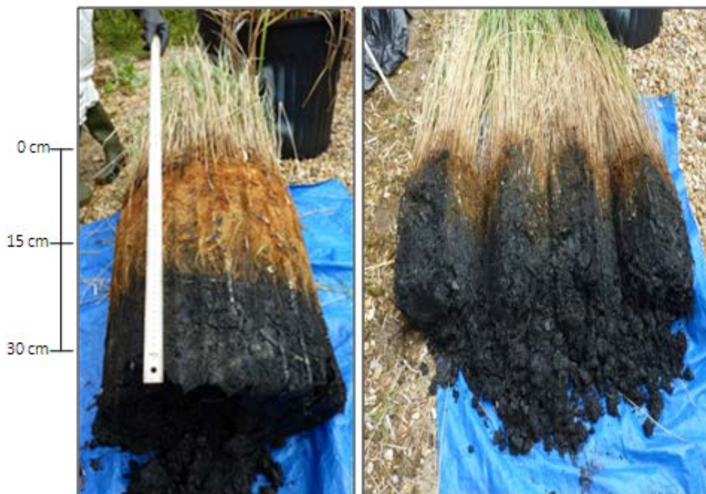
Plate 10. Dismantled mesocosm showing the brown oxygenated, densely rooted sides, H. Pinchin, August 2010.
