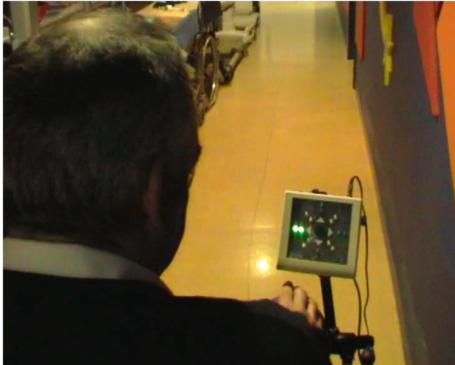
Figure 7.20. A prototype direction scanner coupled with SCAD sensors on a wheelchair detected the walls and objects in the path of travel and provided electronic steering guidance
