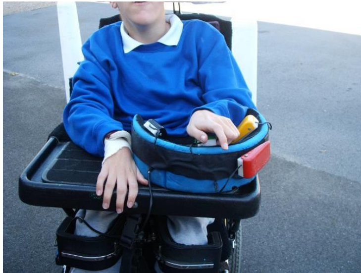
Figure 3.13 Horseshoe surround switches
