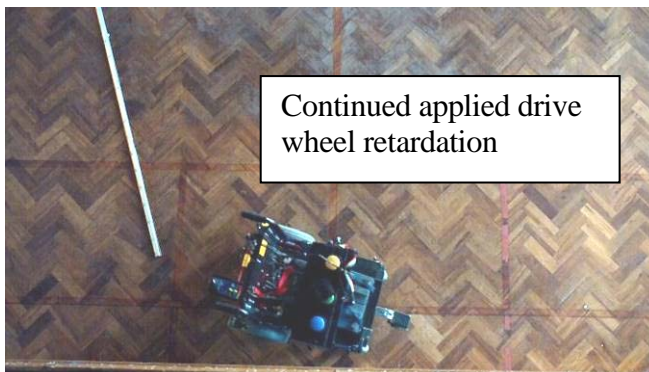
Phase 4 Wheel retardation was reduced as the collision angle became less than at phase 2
