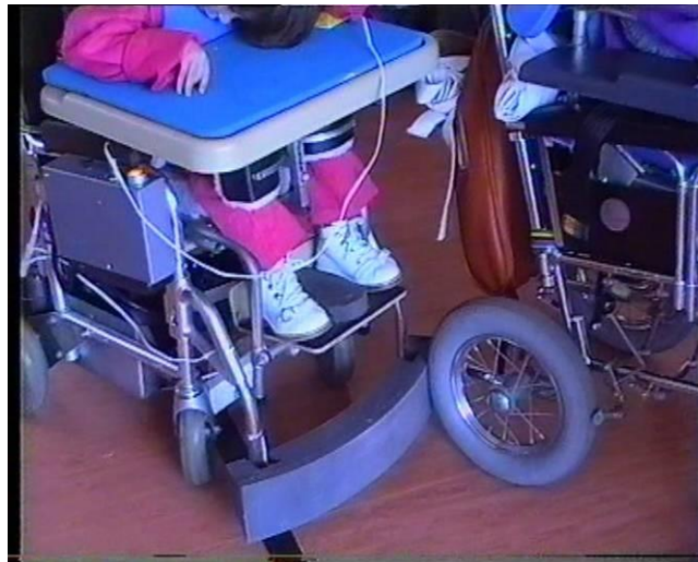
Figure 9.1 A young driver using a track guided wheelchair fitted with a prototype mechanical bumper
