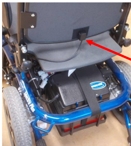
Figure 12.3 The testable gyro based anti-veer system
