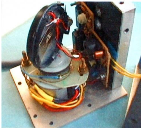
Figure 8.21 Loose transducer twin wire connections
