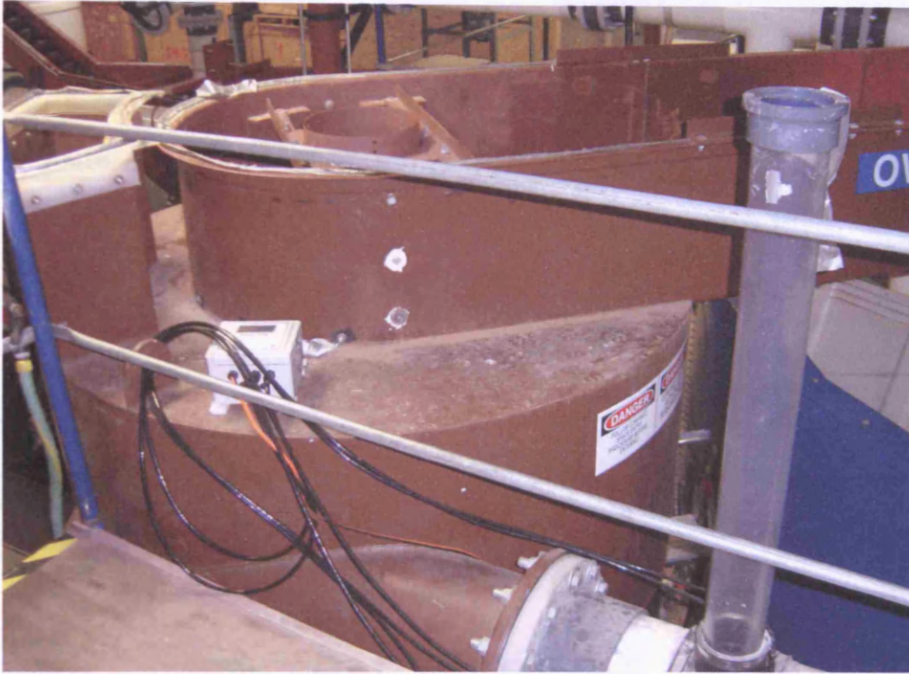
Figure H1. Photograph showing the position of the stand pipe used for introducing the particles into the Grit King ® .
