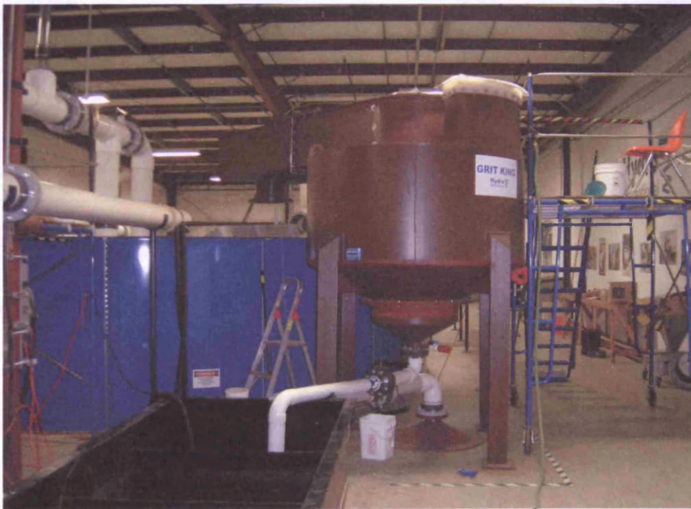
Figure H2. Photograph showing the rear of the Grit King ® and the underflow pipe used for removing the particulates.
