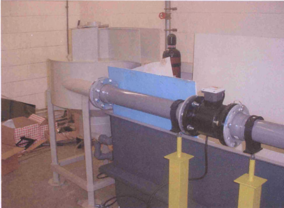
Figure B1. The 0.75m diameter Grit King ® in the laboratory at Cardiff University.
