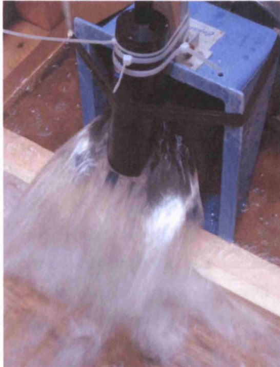
Figure 9-5. (Provided by Ian Guymer ©2004). SCUFA placed adjacent to the underflow.
