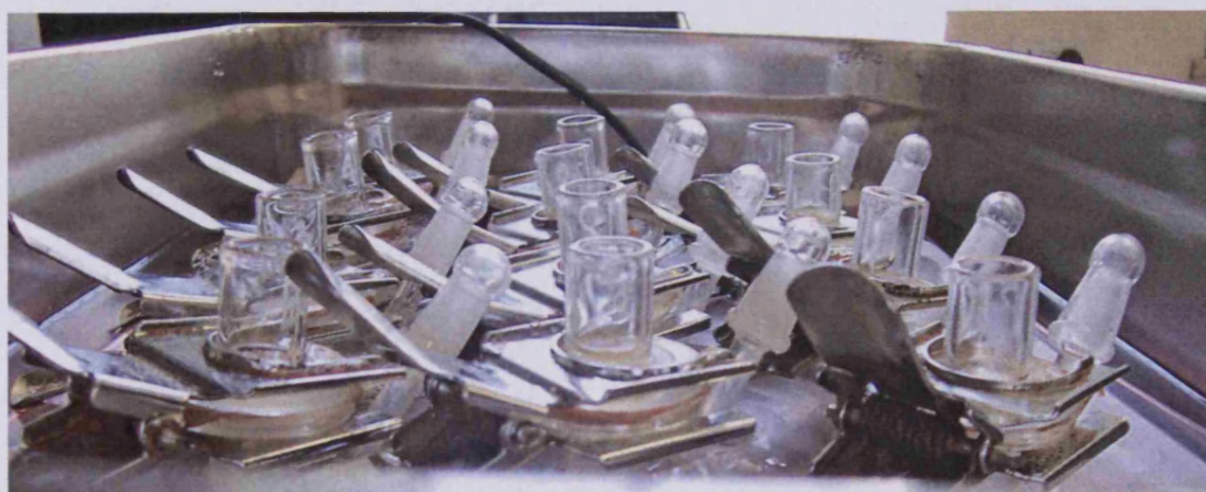
Figure 2.2 Set of 12 diffusion cells in water bath
