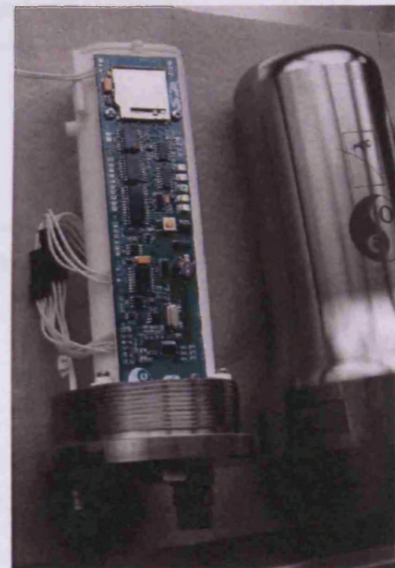
Figure 2.6 Node electronics and pressure case housing manufactured at Cardiff University, UK.
