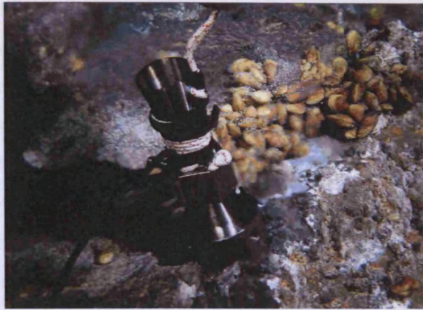
Figure 7.8 Sensor-head deployed on a mussel assemblage on Menez Gwen (MAR).
