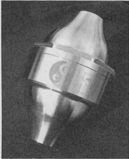
Figure 2.3 Titanium fluid sampling bottle manufactured at MEC, Cardiff University, UK.
