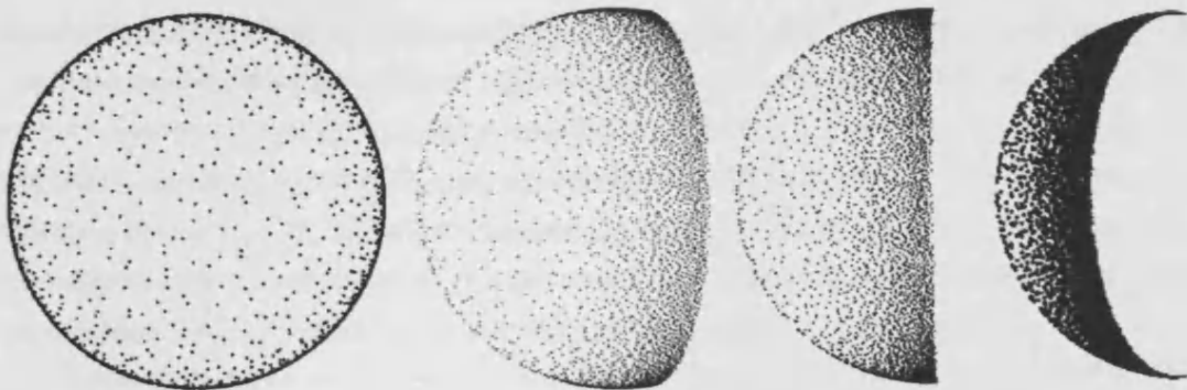
Figure 7.6: Silhouette enhancement with viewpoint dependent rendering: The left-most image shows a sphere from the rendered viewpoint. The remaining three images show the sphere from different angles, whilst fixing the view dependent rendering direction to that of the first image (in order to demonstrate the varying point density).
