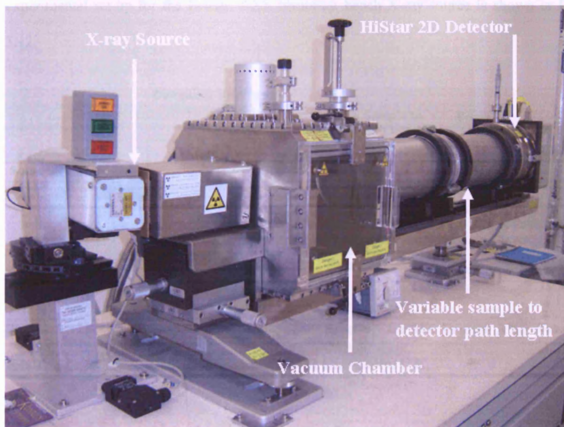
Figure 3.11: An image of the Bruker AXS NanoStar small angle X-ray scattering facility at Cardiff University, U.K.
