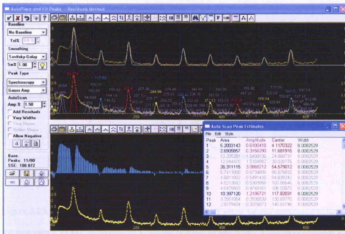
Figure 3.14: A screenshot from PeakFit software. A two-dimensional diffraction pattern obtained from rat-tail tendon has been converted into a one-dimensional linear trace and transferred into the PeakFit software. The peaks observed correspond to the meridional reflections on the diffraction pattern. The software enables users to fit the peaks and obtain parameters such as peak intensity, position and the full width half maximum (FWHM).
