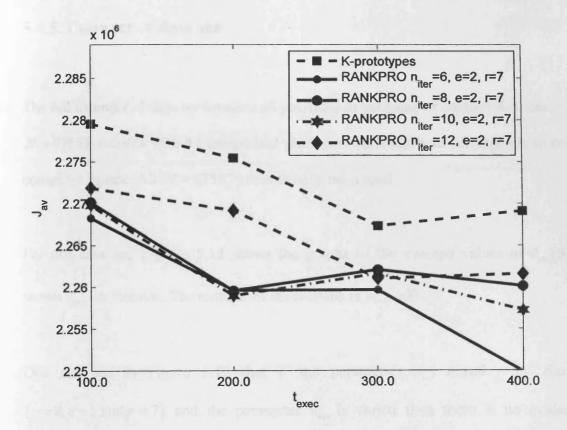
Figure 5.11: The average values of  $J_{av}(S)$  vs.  $t_{exec}$  for Covertype data set. Comparison of the k-prototypes algorithm and the RANKPRO algorithm with different values of  $n_{iter}$ ,  $n_{iter} = 6$ , 8, 10 and 12, while other parameters are constant: n = 9, e = 2, and r = 7.
