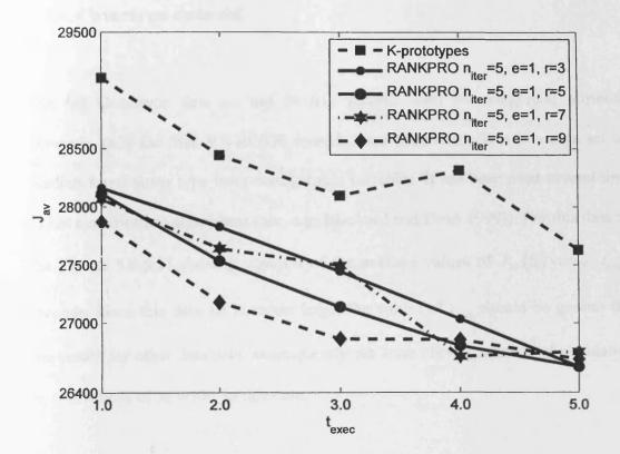
Figure 5.8: The average values of  $J_{av}(S)$  vs.  $t_{exec}$  for Shuttle data set. Comparison of the k-prototypes algorithm and the RANKPRO algorithm with different values of  $n = 4 \div 10$  and correspondingly with different values of  $r = 3 \div 9$ , (r = n - e), and fixed parameters  $n_{iter} = 5$  and e = 1.
