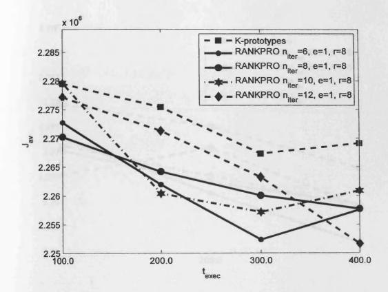
Figure 5.9: The average values of  $J_{av}(S)$  vs.  $t_{exec}$  for Covertype data set. Comparison of the k-prototypes algorithm and the RANKPRO algorithm with different values of  $n_{iter}$ ,  $n_{iter} = 6$ , 8, 10 and 12, while other parameters are constant: n = 9, e = 1, and r = 8.
