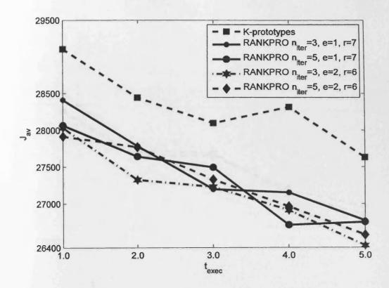
Figure 5.6: The average values of  $J_{av}(S)$  vs.  $t_{exec}$  for Shuttle data set. Comparison of the k-prototypes algorithm and the RANKPRO algorithm with the following parameters: (i)  $n_{iter} = 3$ , e = 1, r = 7 and n = 8, (ii)  $n_{iter} = 5$ , e = 1, r = 7 and n = 8, (iii)  $n_{iter} = 3$ , e = 2, r = 6 and n = 8, and (iv)  $n_{iter} = 5$ , e = 2, r = 6 and n = 8.
