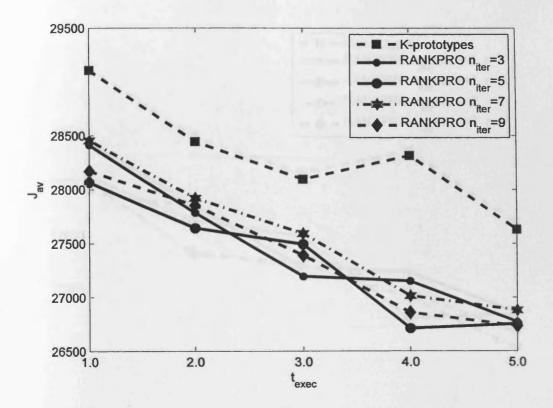
Figure 5.5: The average values of  $J_{av}(S)$  vs.  $t_{exec}$  for Shuttle data set. Comparison of the k-prototypes algorithm and the RANKPRO algorithm with different values of  $n_{iter}$ ,  $n_{iter} = 3, 5, 7$  and 9, while other parameters are constant: n = 8, e = 1, and r = 7.
