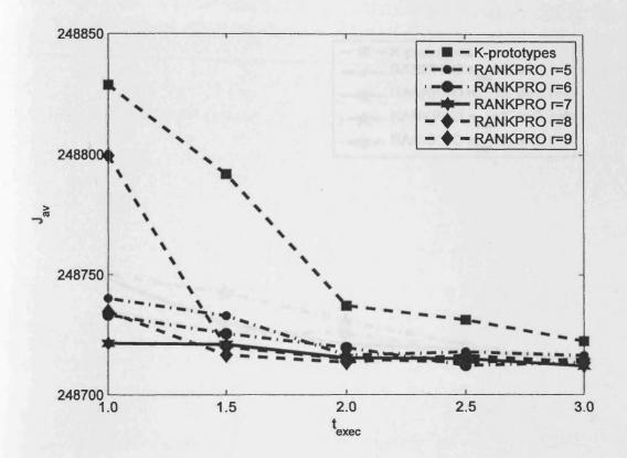
Figure 5.2: The average values of  $J_{av}(S)$  vs.  $t_{exec}$  for ADULT data set. Comparison of the k-prototypes algorithm and the RANKPRO algorithm with the following parameters: (i)  $n_{iter} = 3$ , e = 1, r = 7 and n = 8, (ii)  $n_{iter} = 5$ , e = 1, r = 7 and n = 8, (iii)  $n_{iter} = 3$ , e = 2, r = 6 and n = 8, and (iv)  $n_{iter} = 5$ , e = 2, r = 6 and n = 8.
