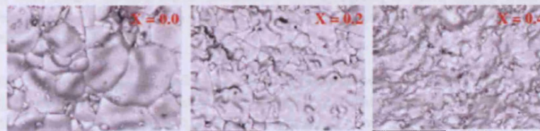
Fig. 2: Backscattered scanning electron micrographs for the \text{CoGa}_x\text{Fe}_{2-x}\text{O}_4 system ( x = 0.0, 0.2, 0.4 )
