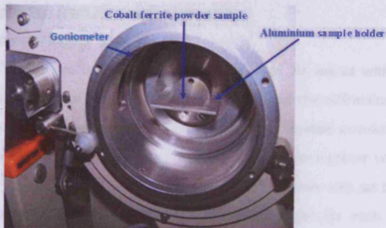
Fig. 5.6: Cobalt ferrite powder sample in the Goniometer for X-ray diffraction
