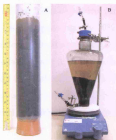
Fig. 2.3: Sediment core and slurry. A: Sediment Core from Tamar Estuary; B: Sediment Slurry Experiment Vessel
