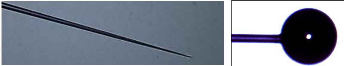
Fig. 6.7 Images of the (a) etched fibre end and (b) formed microsphere at the fibre tip
