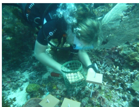
Figure 43: Fixation method of the tiles. Tiles were fixed on a pole 15 cm above the substratum.
