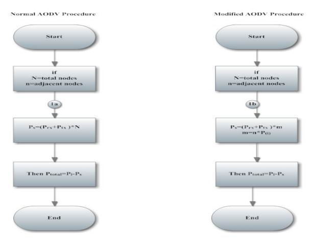
Figure 5.5: Flow chart of the standard AODV and the modified AODV Routing Protocol
