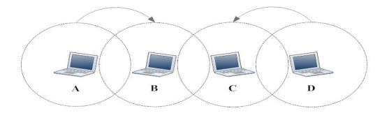
Figure 2.4: An exposed terminal problem in a MANET
