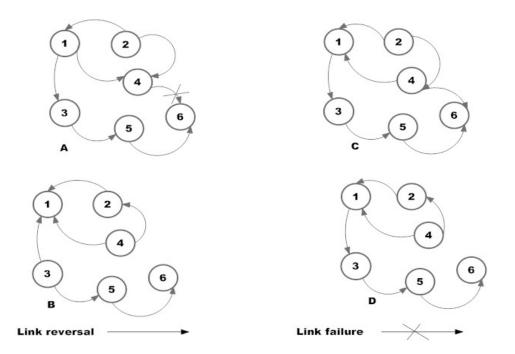
Figure 2.8: TORA Routing Protocol
