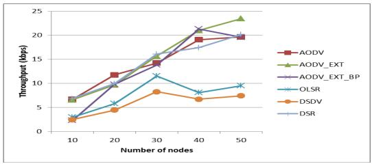
Figure 6.22: Comparison of data throughput for various network sizes (number of nodes)
