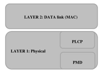
Figure 2.2: Physical Layer Structure
