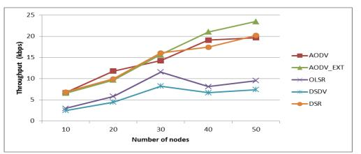
Figure 6.16: Comparison of data throughput for various network sizes (number of nodes)
