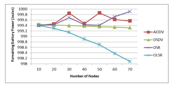
Figure 6.5: Remaining Battery Power versus the number of nodes
