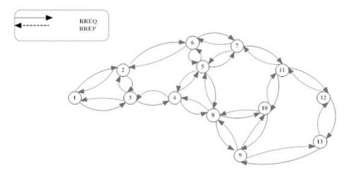
Figure 2.7: A typical AODV network
