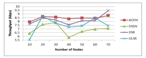
Figure 6.6: Data throughput versus the number of nodes
