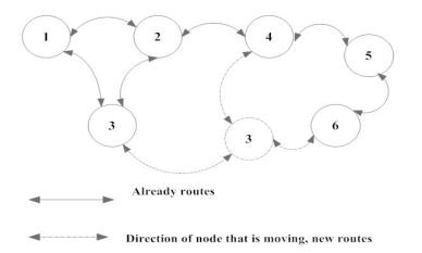
Figure 2.9 An example of the DSDV routing protocol
