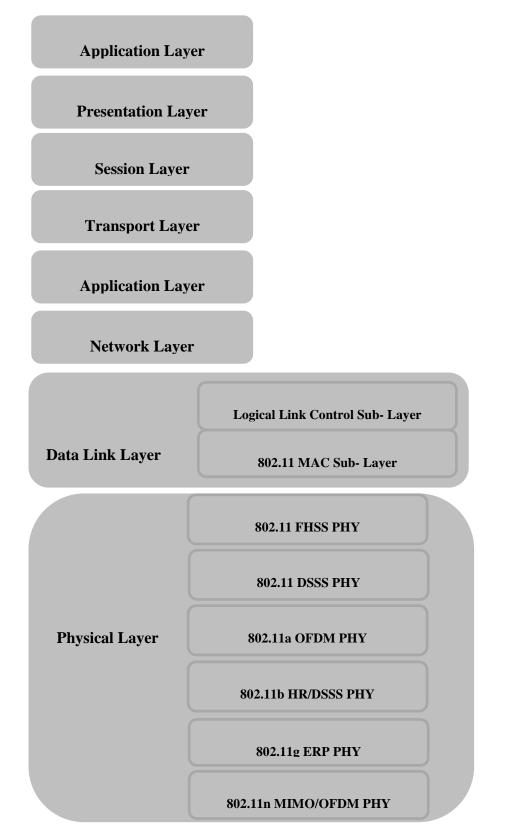
Figure 2.1: MANET (802.11) protocols according to OSI reference model
