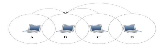
Figure 2.3: A hidden terminal problem in a MANET collision situation
