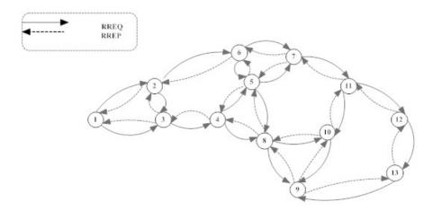
Figure 3.2: A typical AODV network of nodes
