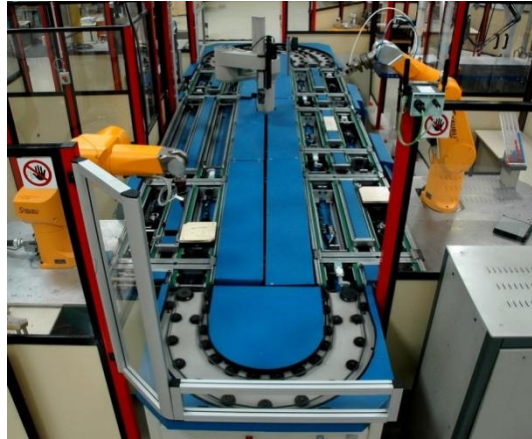
Figure 4-9 The pallet transfer system "SISTRE"
