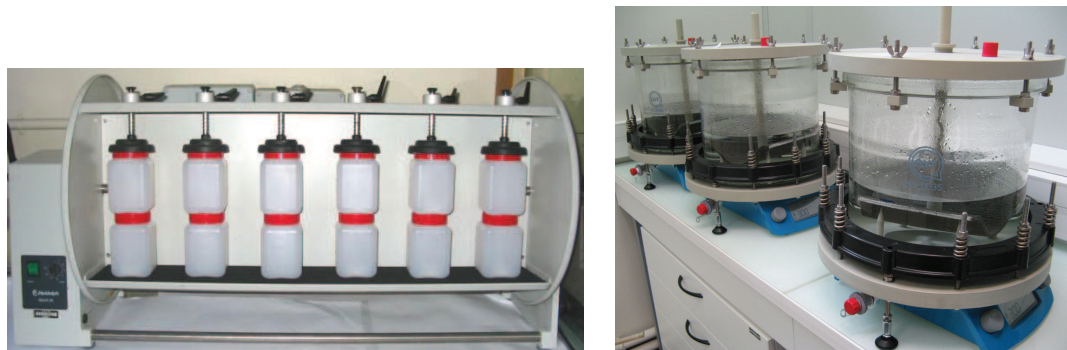
Figure 2.3: ANC installation (left); DSLT reactors (right).
