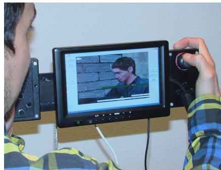
Figure 4.16 – Our hand-held virtual camera device with custom-built dual handgrip rig and button controls, a 7-inch LCD touch-screen.
