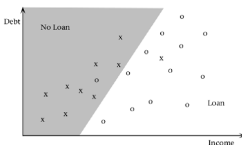
Figure 4.6: A simple linear classification boundary for the loan data set (taken from (Fayyad et al., 1996)).
