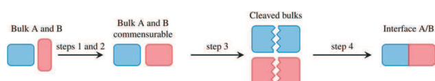
Fig. 1 Successive steps leading to an interface model from two bulk phases A and B.
