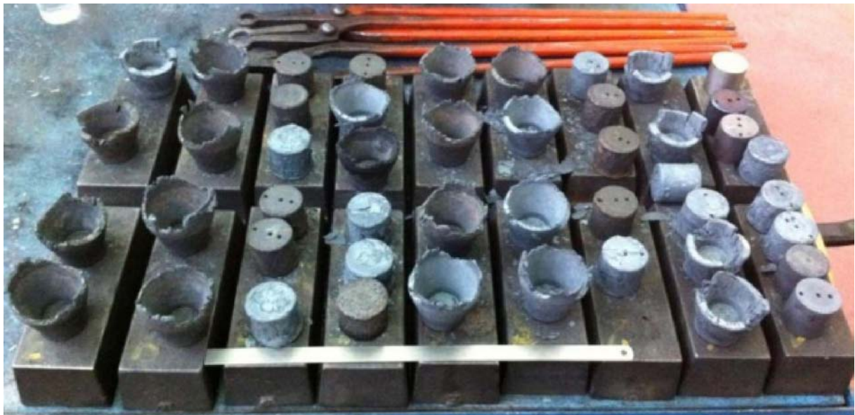
Fig. 4.1. M2 parts obtained by thixoforging process.
