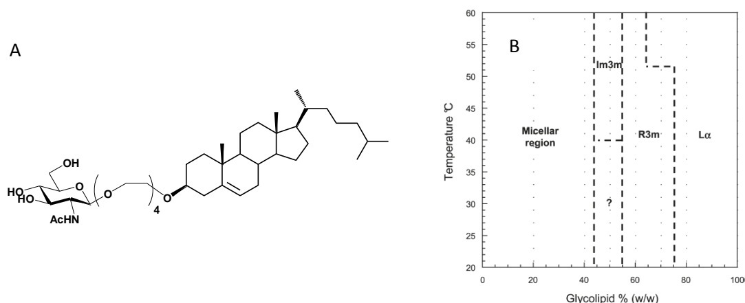
Fig. 4.2: A) Chemical structure of GlcNAc-E 4 -cholesterol and B) its performance in water solution according to the concentration (lines are guides for the eyes, but the error of their positions in terms of glycolipids percentage is \pm 5\% ) [164]
