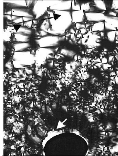
Fig. 1.33: Defect texture of lamellar mesophases with hyperbolic and elliptical lines (black arrows) and oily streaks and fringes around air bubbles (here a Sm A* lamellar phase is shown) [39]
