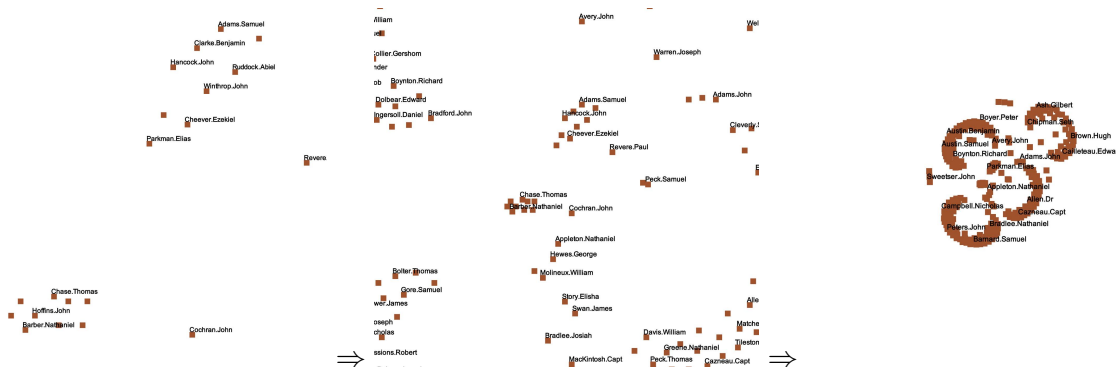
Figure 5.3: Three different levels with “semantic” zooming, for closer on the left to further on the right. The clusters are readable at closer points of view, and aggregate when zooming out.
