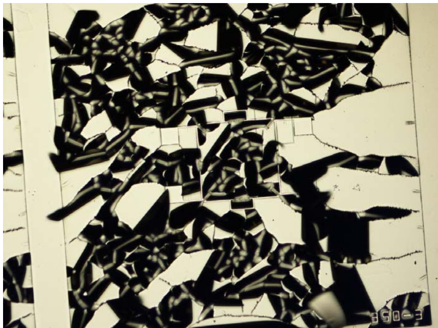
Figure 3.13: Metal peel-off due to large residual stress.
