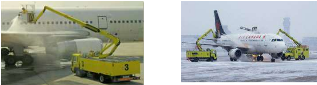
Figure 1.10: On-going de-icing process
