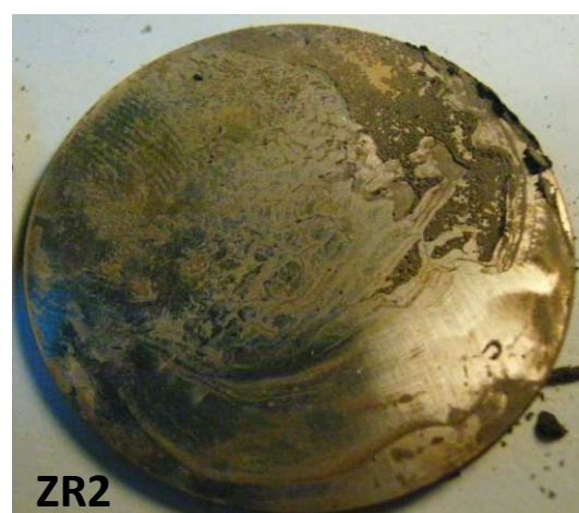
Figure V-108 : disques d'acier inoxydable CI4 (forage horizontal CR6) et ZR2 (forage vertical CR8)
