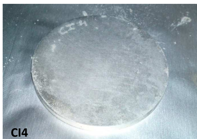
Figure V-108 : disques d'acier inoxydable CI4 (forage horizontal CR6) et ZR2 (forage vertical CR8)
