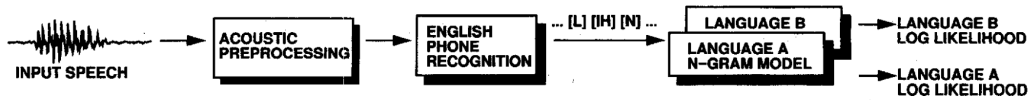
Figure 3.2: The front-end of a PRLM system includes acoustic preprocessing (FE) augmented by a phone recognition step producing a sequence of phone tokens, which is modeled by n-gram language models (back-end). This figure is copied as-is from (Zissman, 1996).
