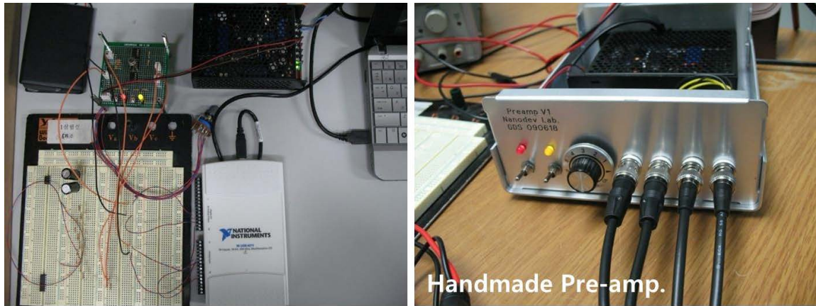
Figure 10. Electrometer systems with NI-DAQ and handmade Pre-amplifier.
