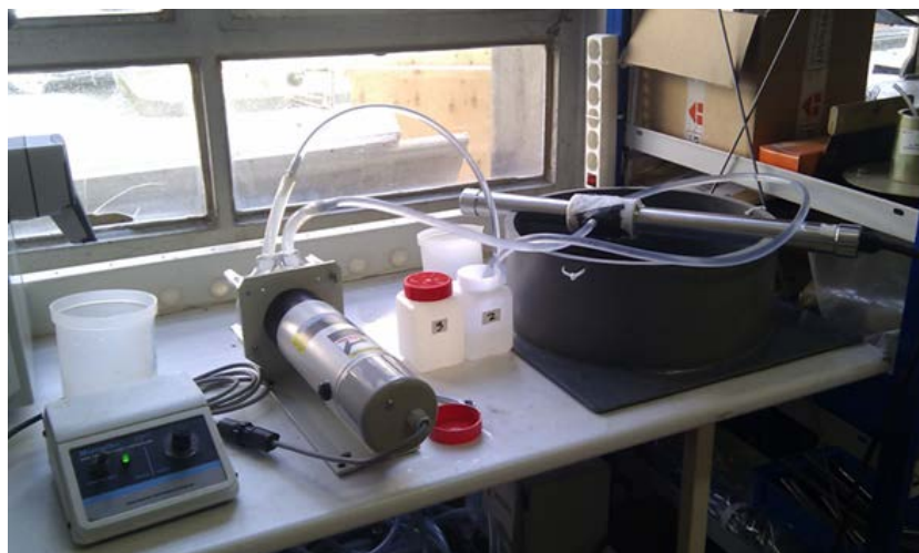
Figure 52: Samples measurement by the S::CAN probe for calibration
