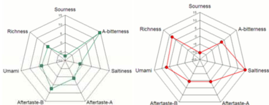
Figure 1.9. Results issue of a taste sensor. The shape of the displayed data gives the user an idea of the taste of beer (in green) and soy sauce (in red). From reference [17]
