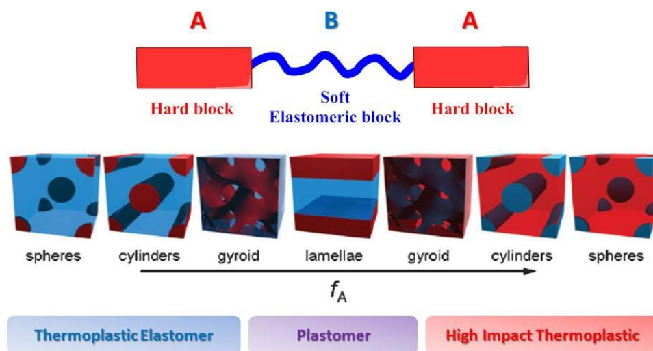
Figure 13.1. Morphologies and mechanical behaviors of block copolymers as a function of the composition
