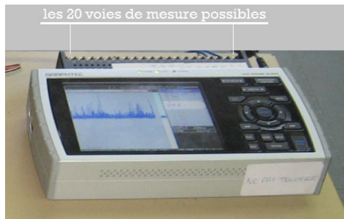
Figure II.37 - La centrale d'acquisition.
