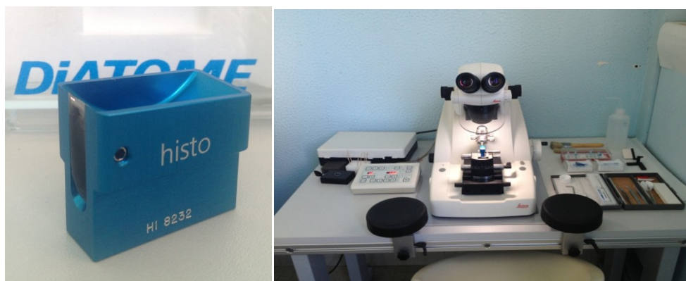
Diamond knife (left) and Leica UC 6 Ultramicrotome system (right)
