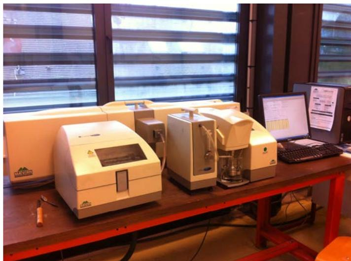
Figure II.6. Photo de granulométrie laser MASTERSIZER 2000, Malvern Instruments Ltd., UK
