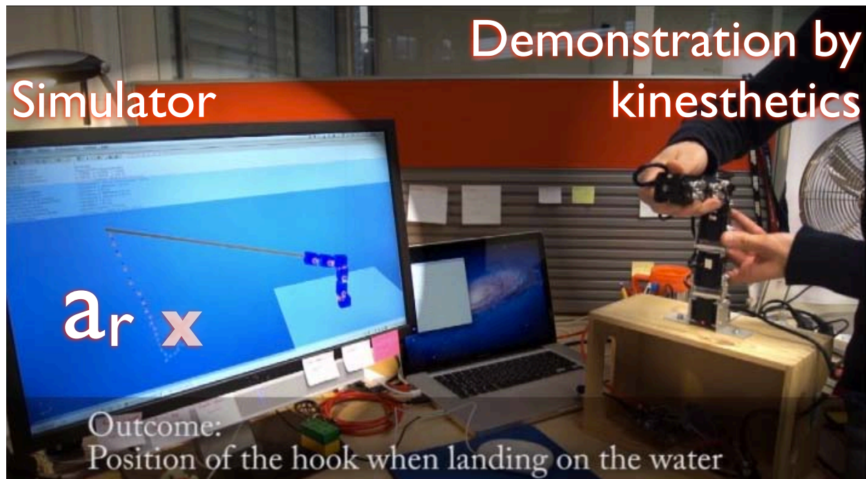
Figure 3.3.2: Demonstration by kinesthetics. A human demonstrator manipulates a physical robot which is connected to a physical simulator.
